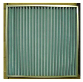
Primary cleanable G3 Filter with aluminium coated double return bent filter frame with no sharp edge, pleated synthetic non woven polyester media. Polyurethane sealing, bonding media to frame.
